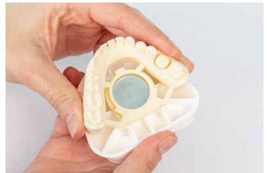
Fig. 16: Detaching the model from the model base plate
