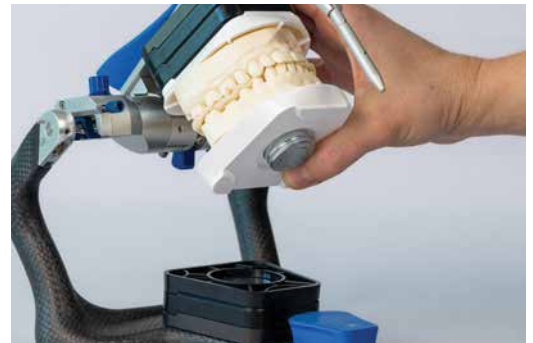
Fig. 17: Standard magnetic pot with Splitex counter plate
