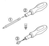
4 With the collet attaching/detaching jig attached onto the torque screwdriver with the sleeve attached, insert the collet attaching/detaching jig into the collet.
