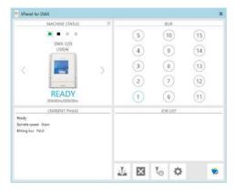
VPanel is an application that allows milling machine operation on a computer screen. It has functions for outputting cutting data, performing maintenance, and making various corrections. It also displays information such as the cutting machine status and errors.
